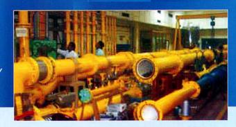
FCRI has established air flow facilities covering areas related to industrial gases. A full-fledged low pressure calibration facility has been in existence since 1989 operating at near atmospheric pressure with flow rates upto 10000 m³/h. Various types of flow meters of sizes upto 400 mm are evaluated with measurement uncertainties, which are in par with international institutions.
