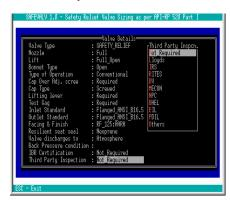
results in a file on a disk or to print it. The output of the software gives computed valve orifice area, selected valve from the database and its characteristics.
