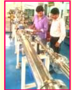
Testing of bulk water meter for Nuclear Fuel Complex Hyderabad
