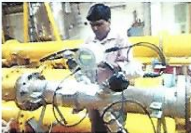
Ultrasonic flow meter under Calibration at AFL
