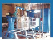
Apart from Hydraulic Performance tests and calibrations, FCRI is involved in evaluating and certifying Flow Products in Special Purpose Test Facilities. Here the performances of the flow products are checked for severe operating conditions as per design to evaluate its life in line with international and national standards. This facility also provide special tests for specific industries like Nuclear and Hydro Power industry, Water distribution systems, Automobile and aerospace industries.
