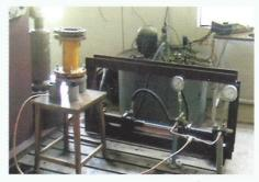
determine leakage of hoses or hose assemblies, the specified proof pressure in accordance with the product standard is applied and the test components are examined during this period for evidence of leakage, cracking, abrupt changes in the dimensions of the component. The online data was logged to the Data Acquisition system continuously.
