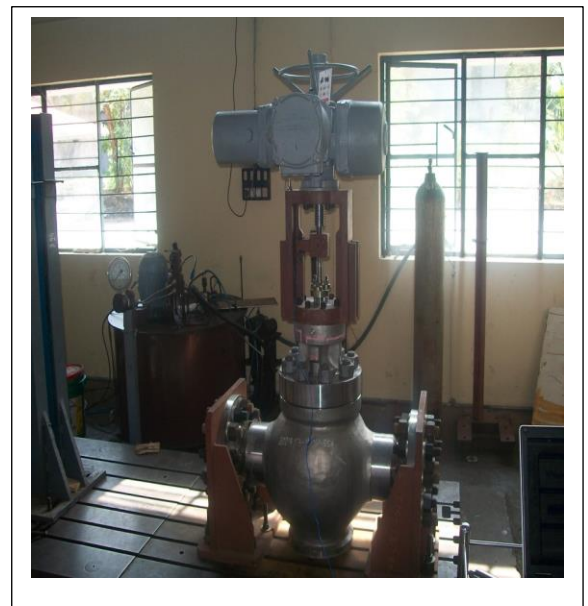
Impact Hammer Testing of control valve
