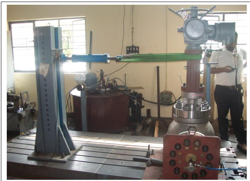
Static load Testing of control valve
