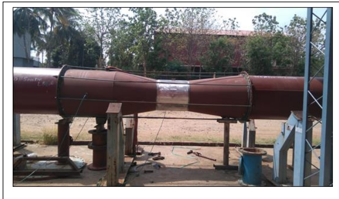
950 mm Venturimeter under calibration at LWFL
