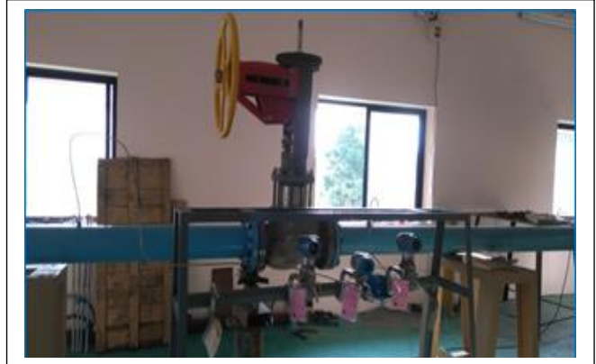
F_L Testing of Globe Valve
