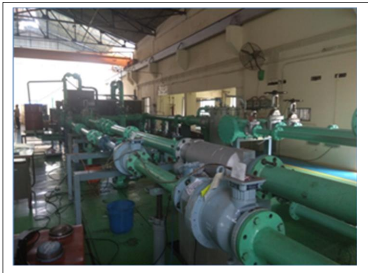
PD Meter under calibration at OFL
