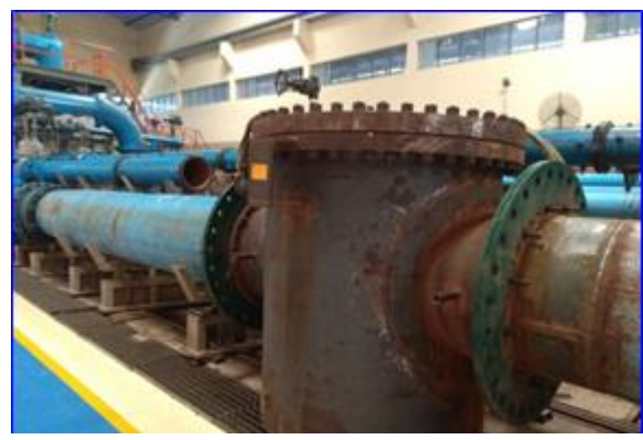
A strainer under test
