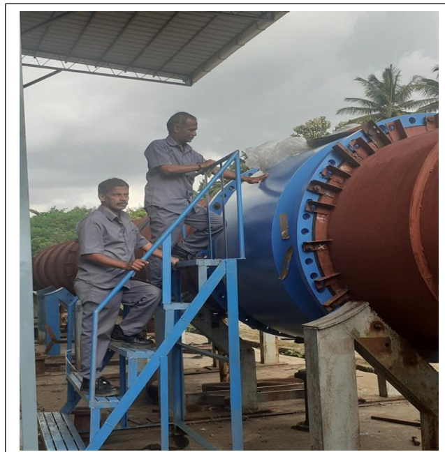
Calibration of Electro Magnetic Flow meter (EMF)
