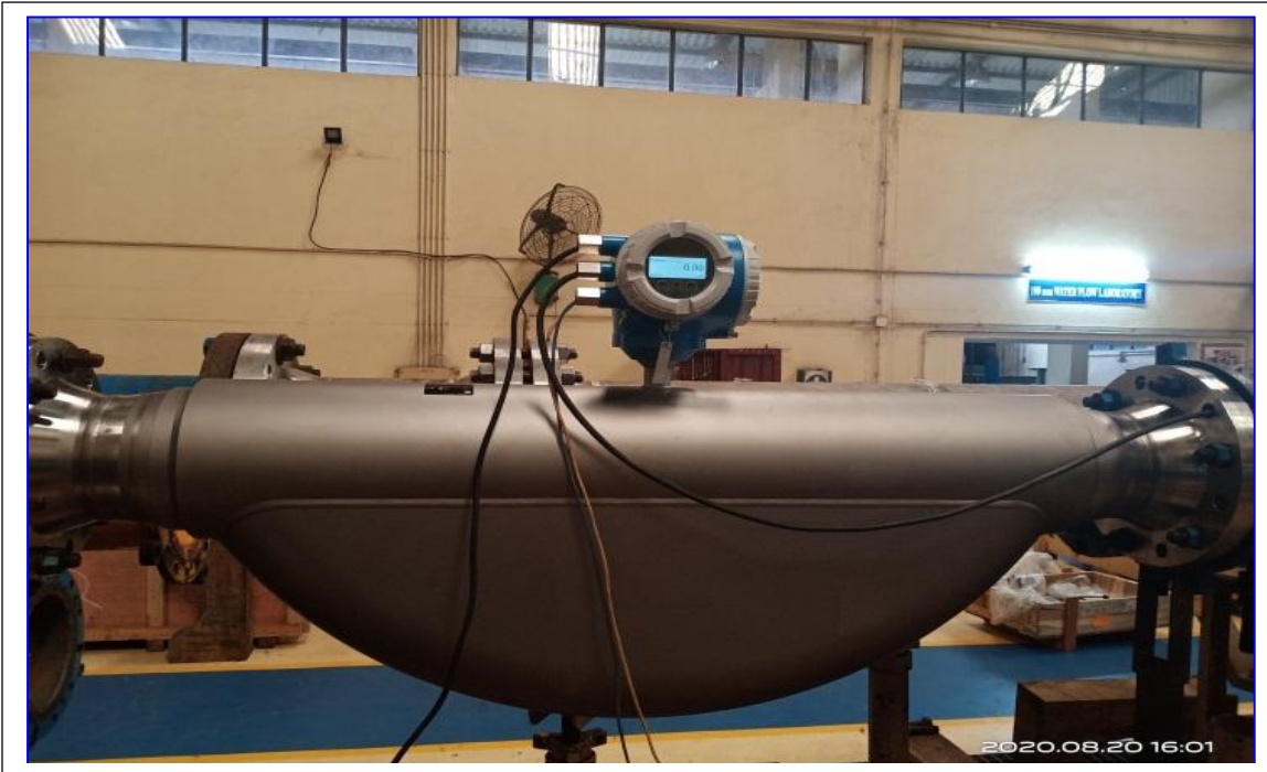
Calibration of mass flow meter at WFL
