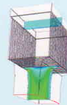
Flow velocity contours in a section of rectangular duct air inlet silencer
