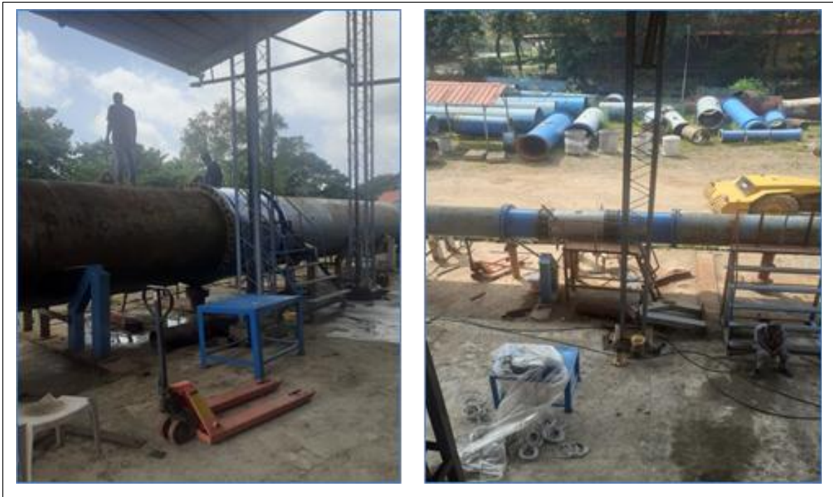
Calibration of 2000mm Electro Magnetic Flow meter (EMF) & 800mm Ultrasonic Flow meter
