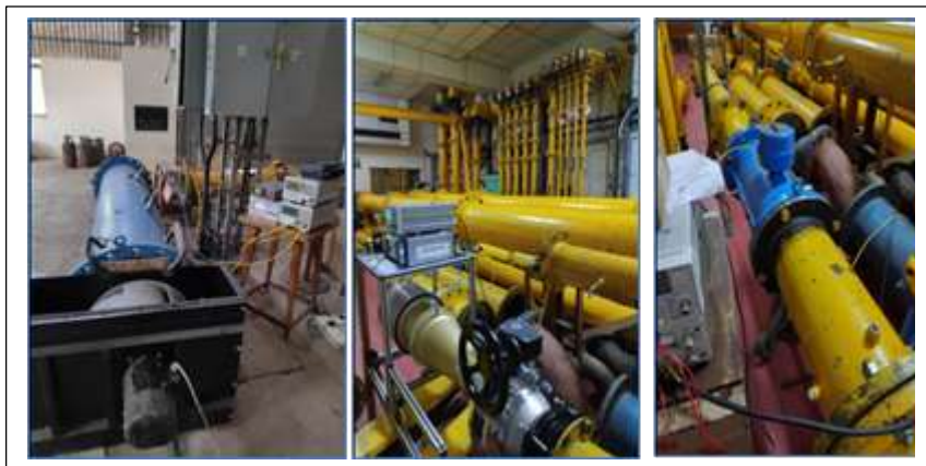
Various Flow Elements being tested at AFL
