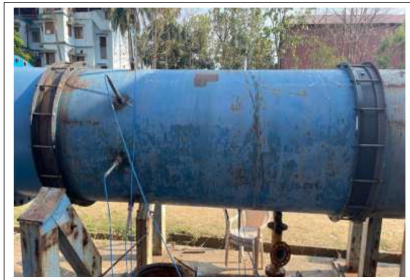
Calibration of 1200mm USFM at LWFL
