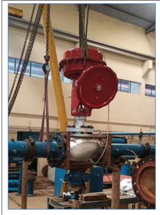
Testing of 8" angle valve at WFL
