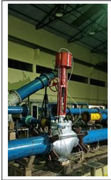
Testing of Control Valve at WFL
