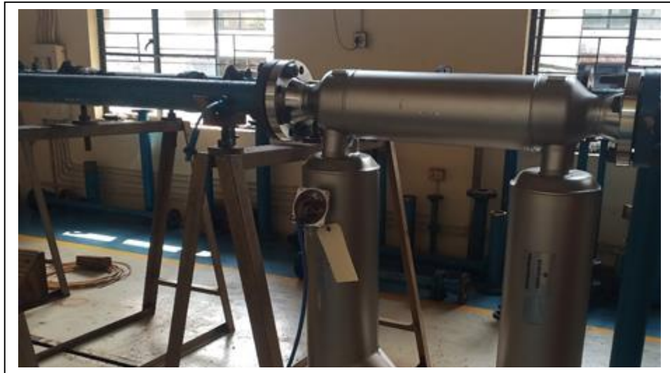
Mass Flow Meter Calibration at WFL
