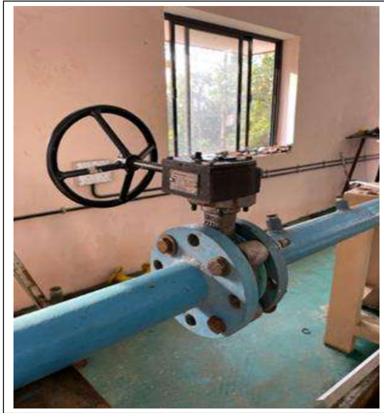
Test on Butterfly Valve in Valve Cavitation and Research Centre of FCRI.
