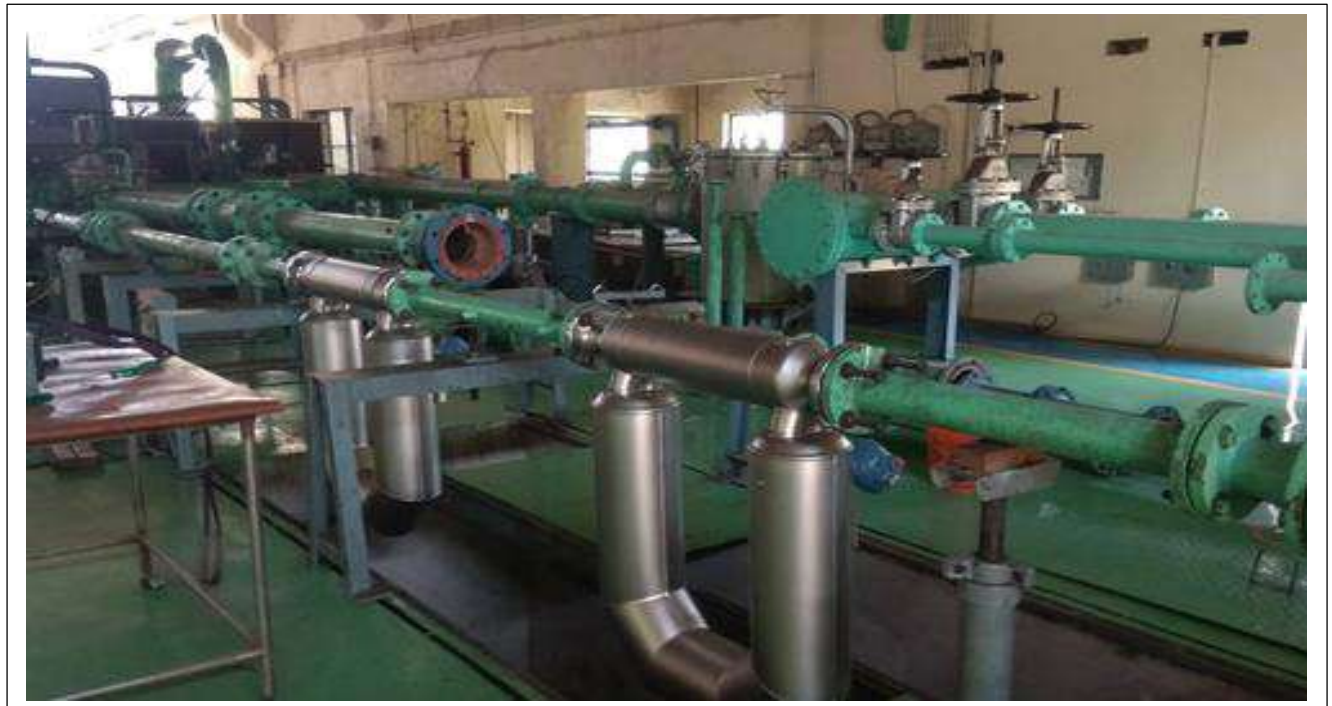
Calibration of 6" mass flow meter at OFL
