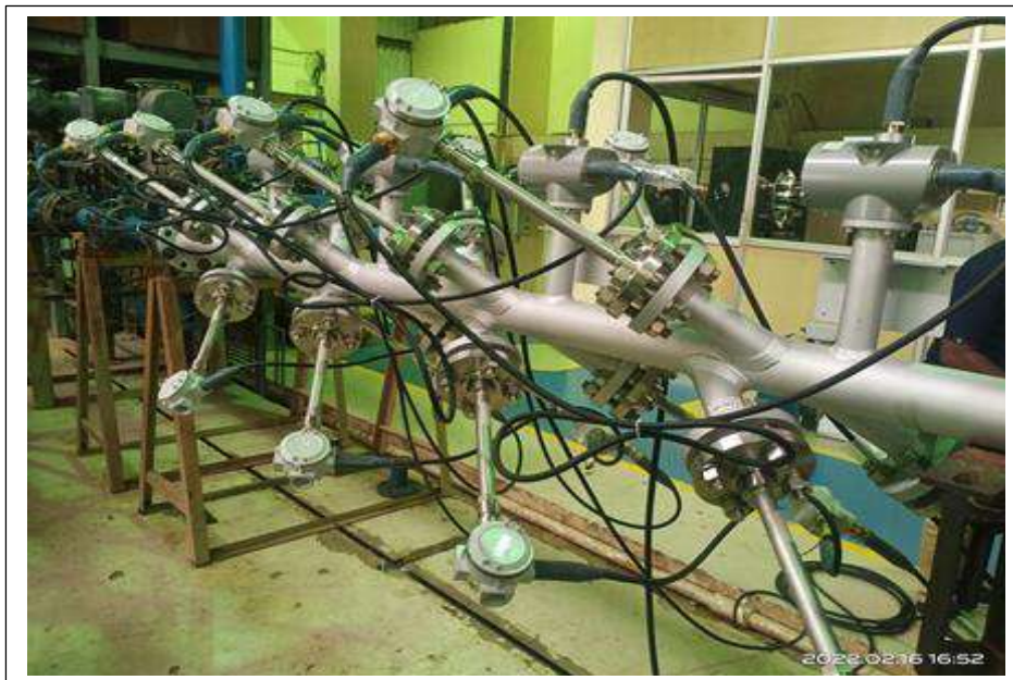
Calibration of multipath insertion type ultrasonic flow meter
