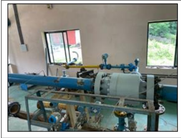
Testing of high pressure 3 way by-pass valve at VCRC
