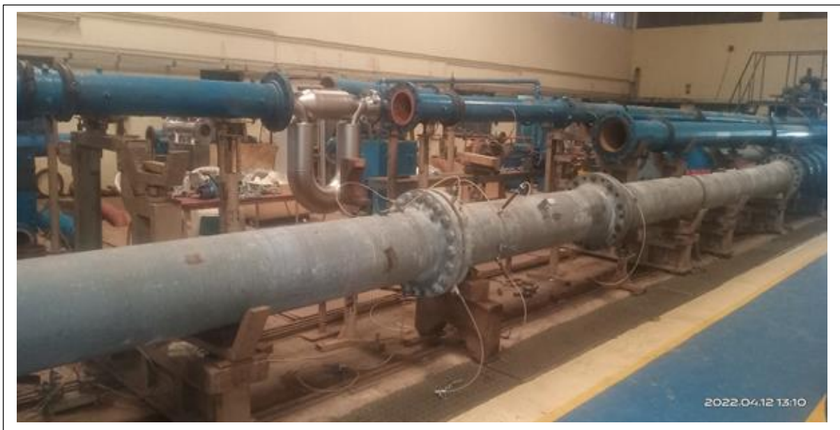
Calibration of throat tap Flow Nozzle of size 16" at WFL
