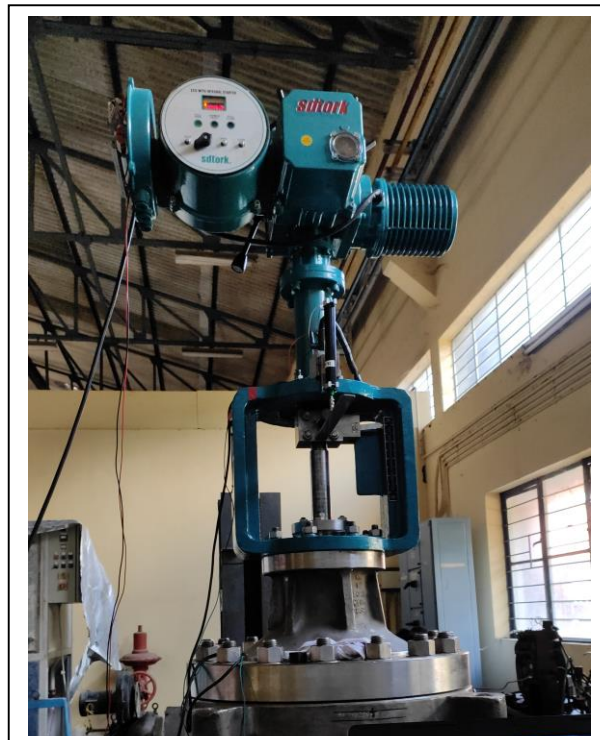
Dynamic Response Testing of 14" Control Valve
