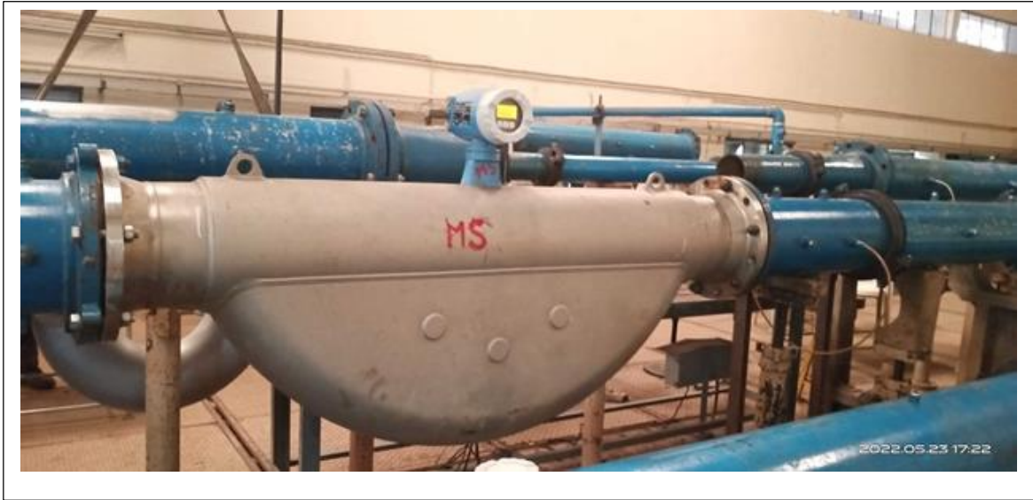
Calibration of mass flow meter (Size 10") at WFL
