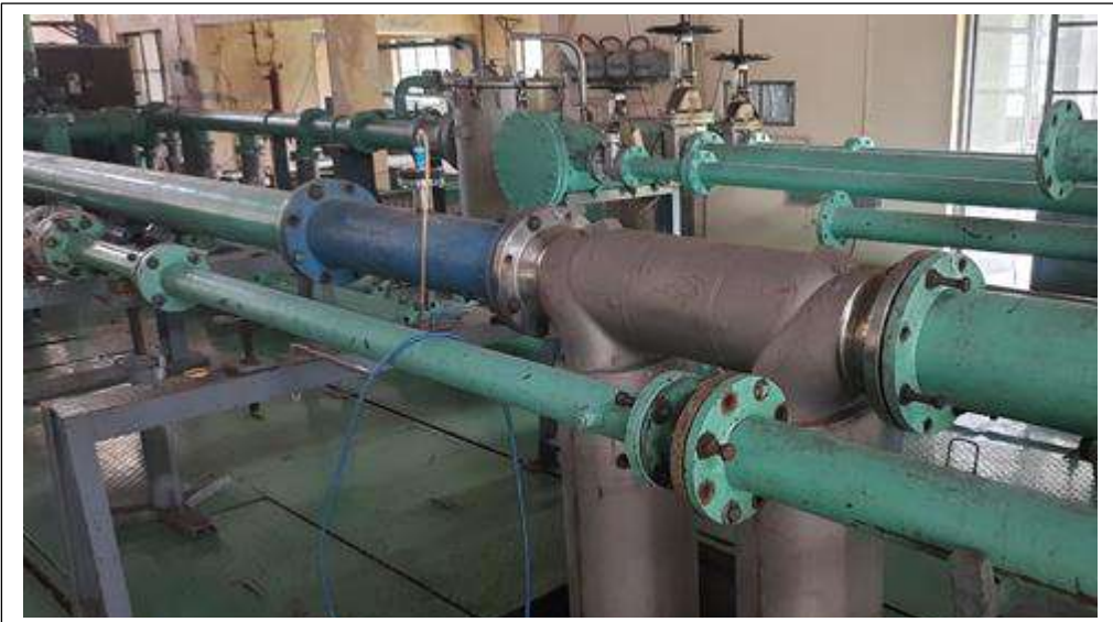
Calibration of mass flow meter of size 6" at OFL
