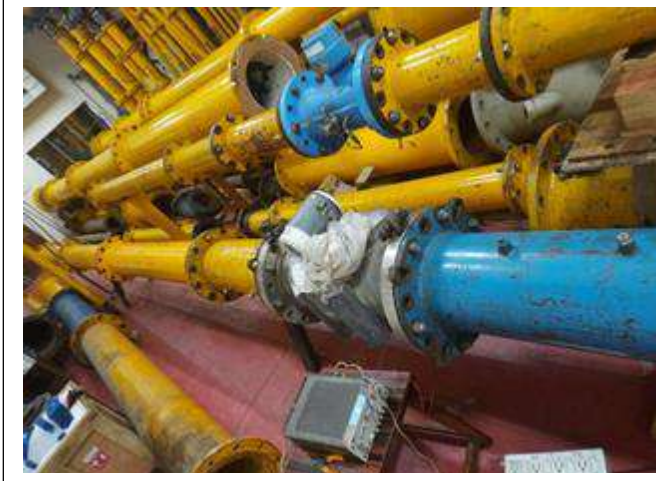
Calibration of flow meters at Air Flow Laboratory
