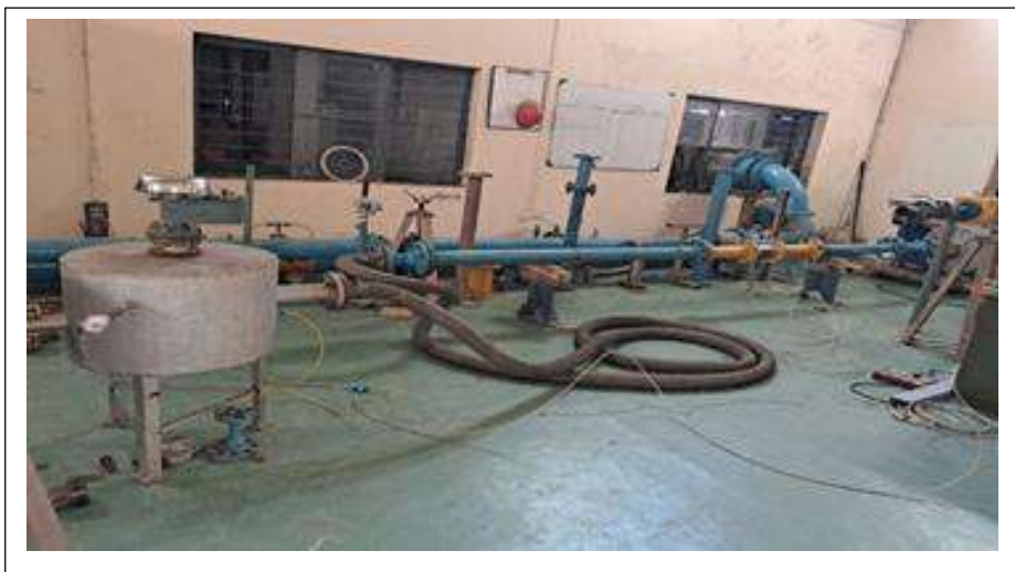
Testing of 2" Breather Valve at HPATF
