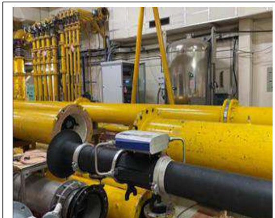
Calibration of flow meters at Air Flow Laboratory
