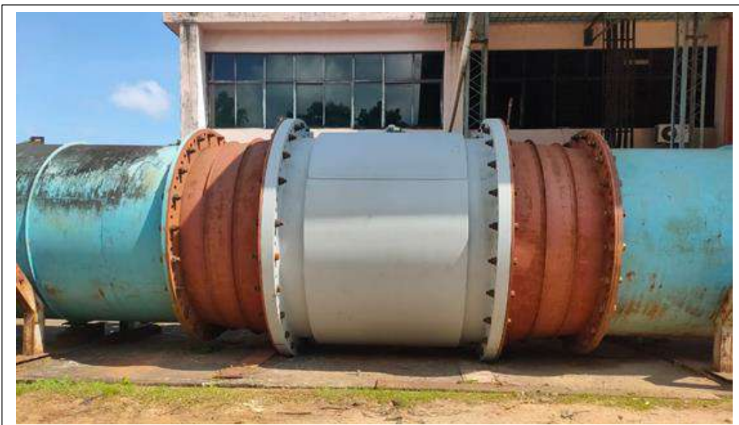
Calibration of 3000 mm Electromagnetic flow meter at LWFL
