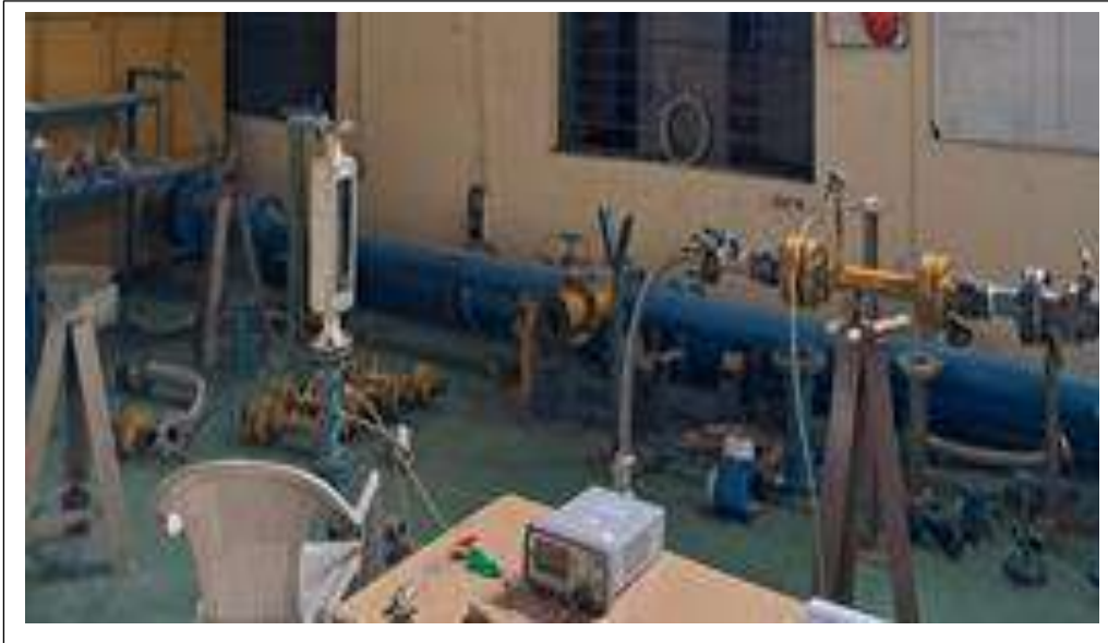
Calibration of Rota meter at HPATF
