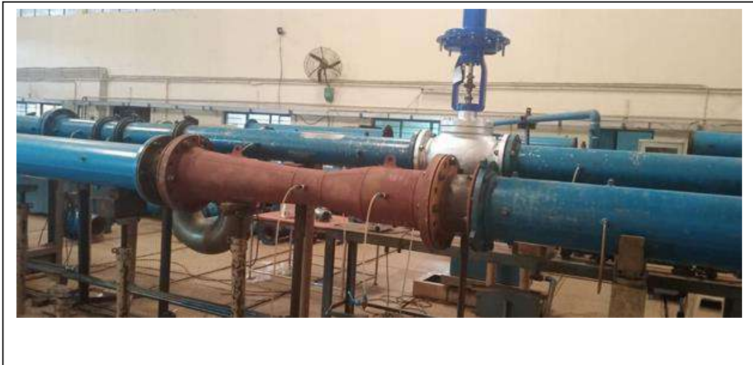
Calibration of 24" Venturimeter at WFL
