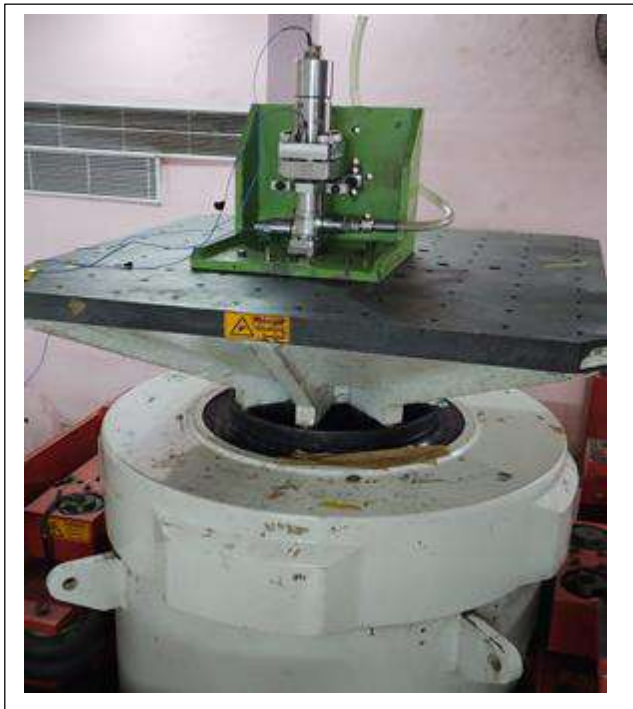
Vibration testing of Valve
