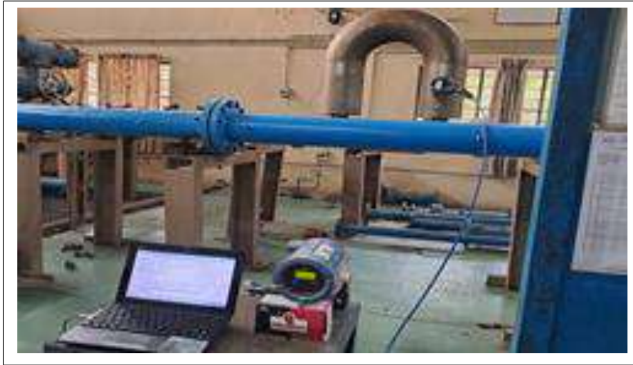
Calibration of Mass Flow Meter at HPATF
