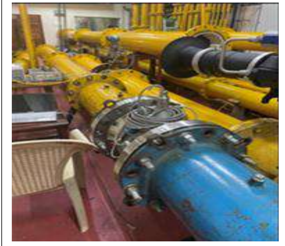
Calibration of flow meters at Air Flow Laboratory
