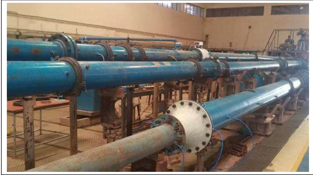
Calibration of Flow Nozzle of size 20" x 10" at WFL
