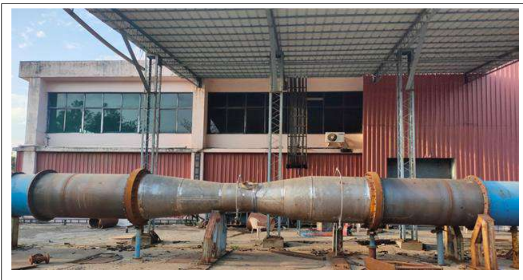
Calibration of 1300 mm Venturi meter at LWFL
